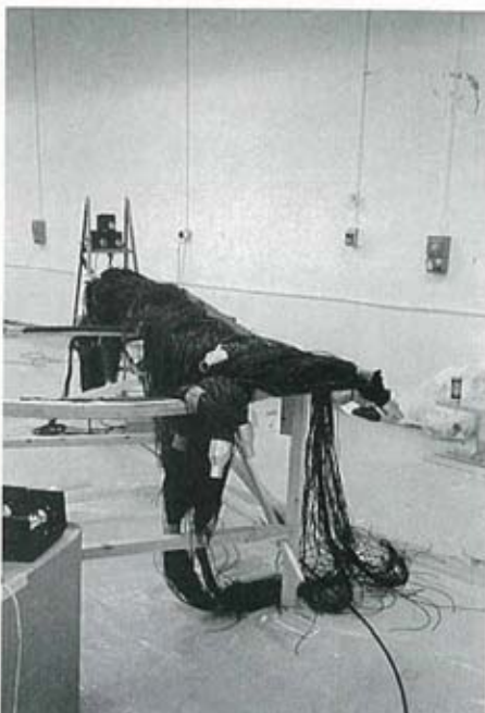
One of the fibre optic signs; each message contains some 1,500 individual fibre optics.
